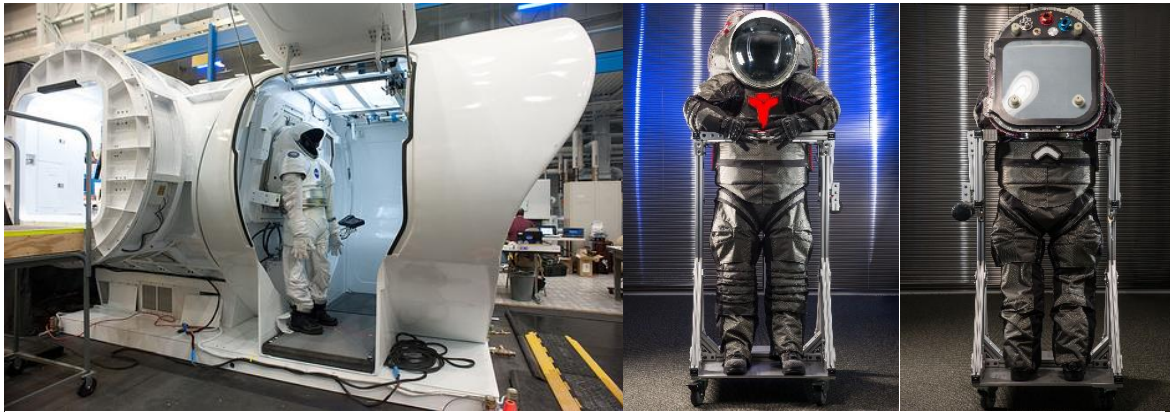
Figure 3 NASA Left: Crew Exploration Vehicle Study article and integrated suit port assembly – Right: NASA Z-2 prototype – credit NASA
